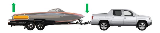
V Drive or rear engine mount boats generally have a fuel tank located above the axle group and as a result the fuel level does not affect the Tongue Weight as significantly as centre mount boats.
