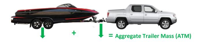
Do not tow the boat with water in the ballast tanks/bladders or excessive gear/lead etc... Always empty the contents or the tongue weight will be incorrect and GTM, ATMs and/or other limits may be exceeded. This may also result in the improper distribution of the weight on the trailer.
