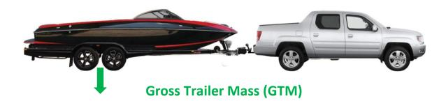
You must ensure that the total weight of the boat, engine, gear and trailer do not exceed the maximum permitted GTM at the wheels and the maximum permitted ATM overall.
