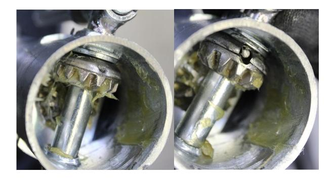
Rotate the securing plate to expose the pin in the shaft of the handle.
