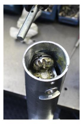
Once the pin is out you can pull the shaft out as shown in the picture.
