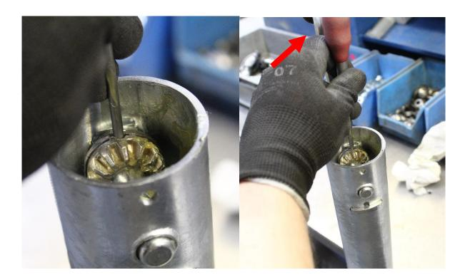
When the pin is exposed rotate the handle to the upright position (shown with the red arrow) then hit the pin with a punch tool to drive it out.
