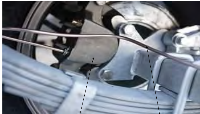
Figure 6b – Hydraulic Disc Assembly (fitted with optional park brake)
